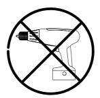
We strongly advise that you do not use Power Tools, such as drills or electric screwdrivers during the assembly as this may cause irreparable damage and will invalidate your warranty.
